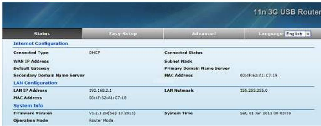
◆ If the *Connected Type* is different, e.g. DHCP, then select **Easy Setup** en select: USB-Wireless adapter
